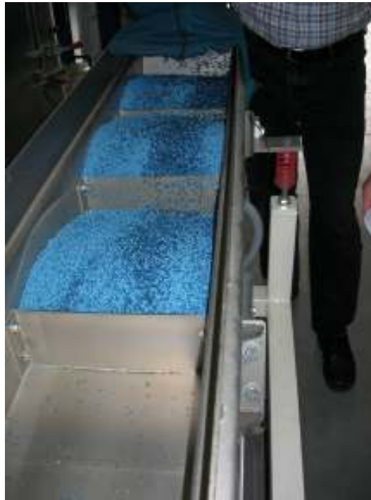
Figure 6 Crystallizing PET granules on vibrating table
